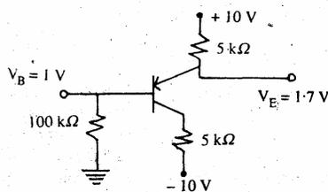
A circuit using the BJT is shown in the above figure, the value of  $\beta$  is
