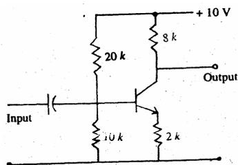
For the circuit shown in the above figure,  $\beta=100$  for the transistor, the transistor will be in
