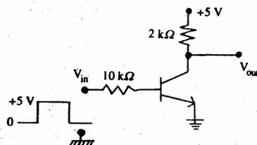
A switch circuit using the transistor is shown in the above figure. Assume  $h_{FE(min)} = 20$  and  $f\tau = 100\text{MHz}$ . The most dominant speed limitation is brought by
