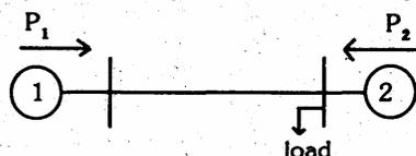
Two power plants interconnected by a tie-line as shown in the above figure have loss formula coefficient  $B_{11} = 10^{-3} \text{ MW}^{-1}$ . Power is being dispatched economically with plant '1' as 100 MW and plant '2' as 125 MW. The penalty factors for plants 1 and 2 are respectively
