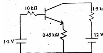
For the circuit shown in the above figure, by assuming  $\beta=200$  and  $V_{BE} = 0.7\text{V}$ , the best approximation for the collector current  $I_c$  in the active region is
