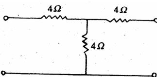
For the circuit shown in the above figure  $h_{11}$ ,  $h_{12}$ ,  $h_{21}$  and  $h_{22}$  are respectively
