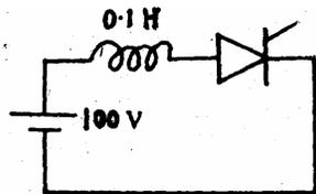
The latching current in the above circuit is 4 mA. The minimum width of the gate pulse required turn on the thyristor is
