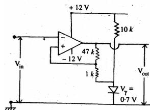
The Schmitt trigger circuit is shown in the above figure. If  $V_{sat} = \pm 10\text{ V}$ , the tripping point for the increasing input voltage will be
