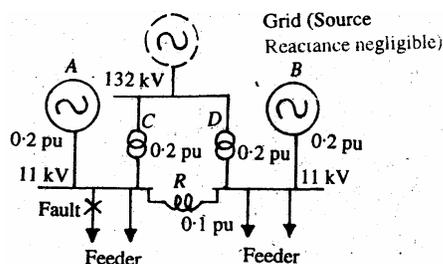
The above diagram shows the layout of a power station having two generators A and B, connected to the 11 kV buses which are also fed through two transformers C and D from a 132 kV grid. The 11 kV buses are interconnected through a reactor R.
