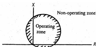
The operating characteristic of a distance relay in the R-X plane is shown in the above figure. It represents operating characteristic of a
