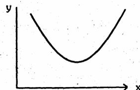
In the 'V' curve shown in the above figure for a synchronous motor, the parameter of x and y coordinates are, respectively
